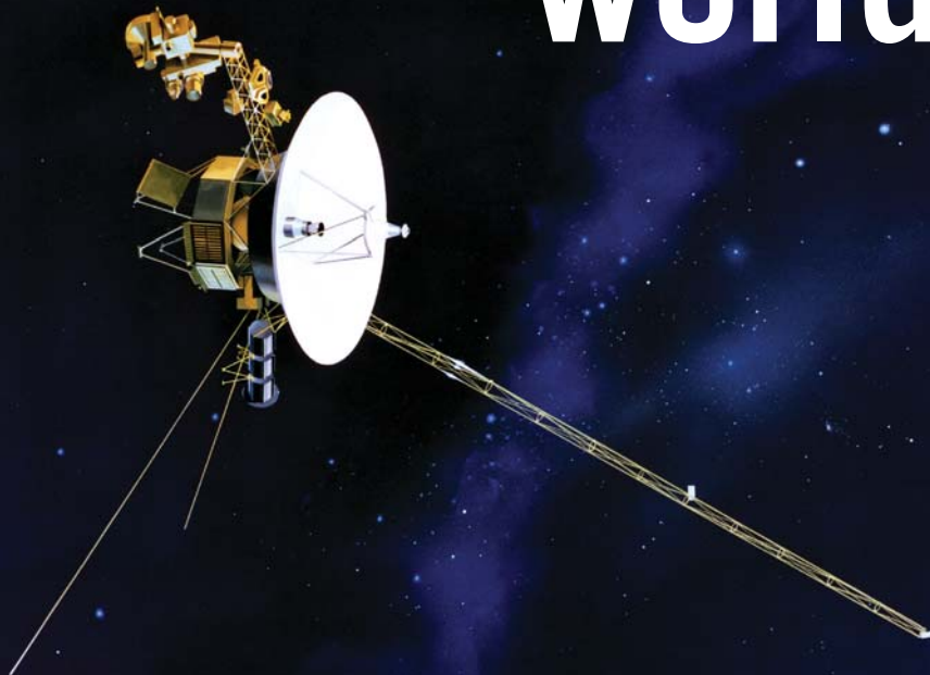
Artist's impression of the Voyager 2 spacecraft showing the communication dish and booms with instruments that measure magnetic fields, energetic particles, plasma, and radio waves.
